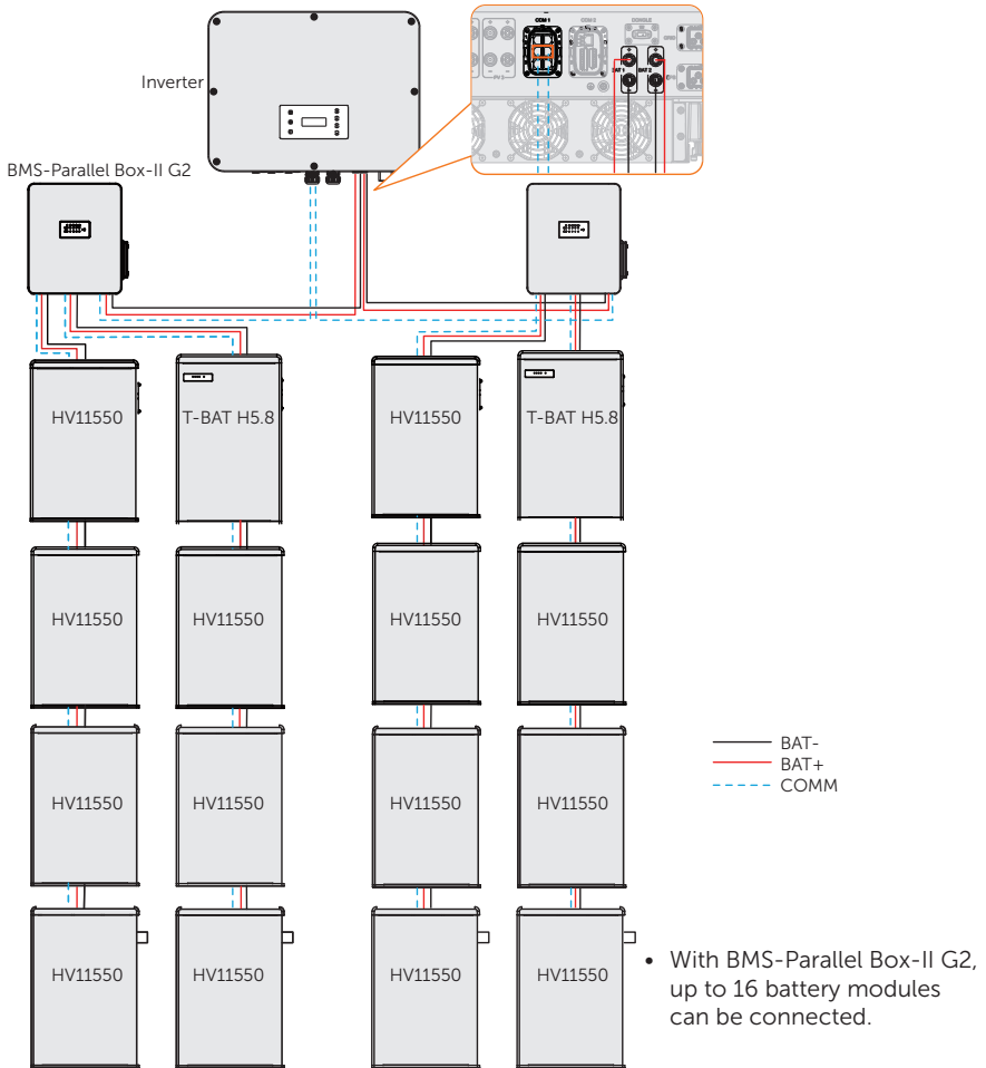
Figure 8-25 Battery connection with BMS-Parallel Box-II G2
